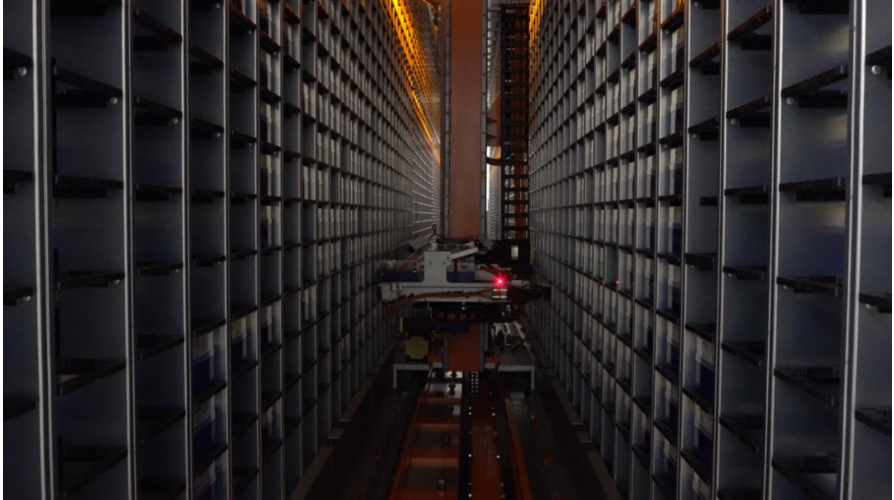
Robot moving newborn blood cards in the automated freezer, Danish National Biobank, Copenhagen, 2018
